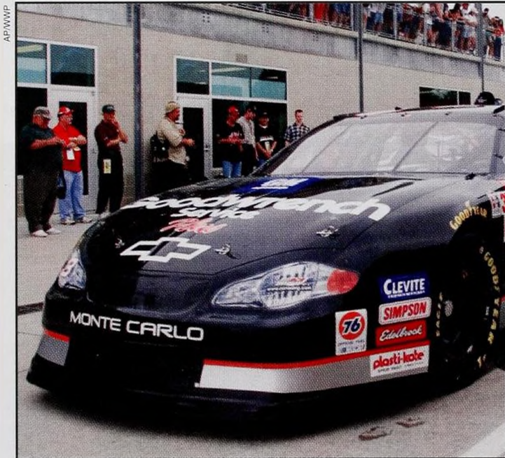
Stock cars are equipped with protective window nets and plastic windshields to prevent injury.
