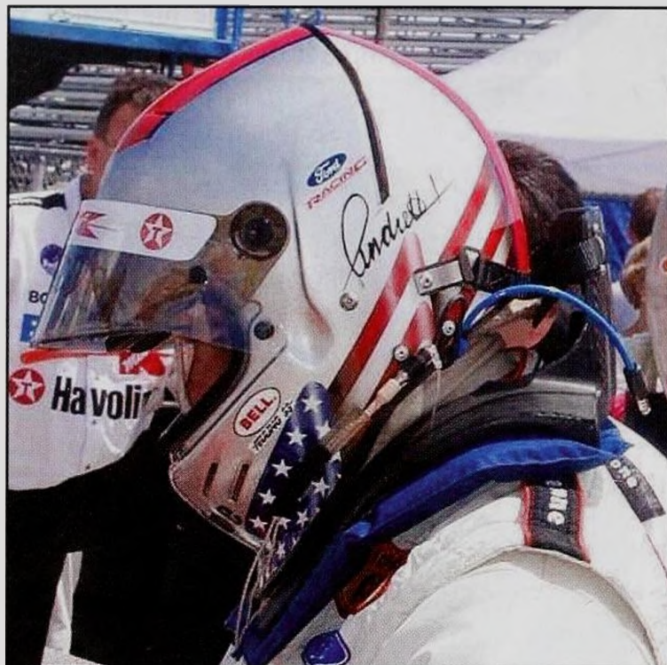
The HANS system protects a driver's head and neck from damage in a crash.
